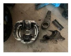
at the piston ripped out. My conclusion is that the first point of failure was the piston itself as the gudgeon pin appeared to have ripped out of the bottom of the piston. If the con-rod or big end had failed first there wouldn't have been a mechanism to cause this damage – i.e. no con-rod, nothing to pull down on the piston.
